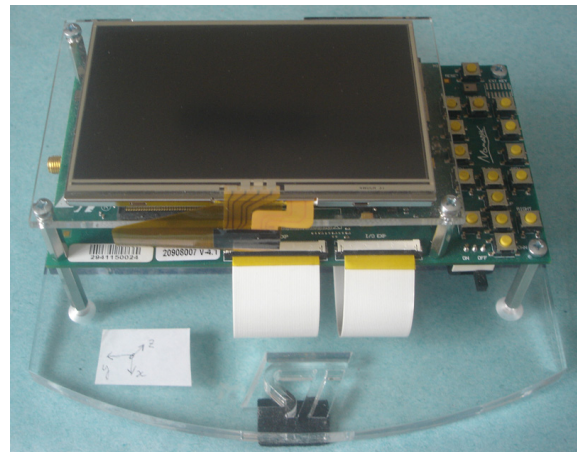
Figure 4: The Nomadik NHK8815 evaluation board.
