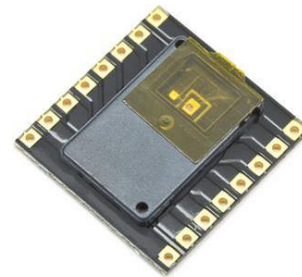
Figure 31: Avago ADNS-3550, an ultra slim motion sensor
