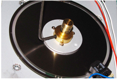
Figure 4: A Vestax VCI-400 jogwheel being disassembled
